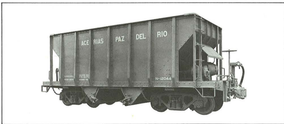
Twin-hopper iron ore cars for Colombia; Gregg-Barber stabilized bogies with Unit brake beams and Timken AP bearings. Capacity: 35 metric tons — 770 cubic feet. Track Gauge: 3'-0".
