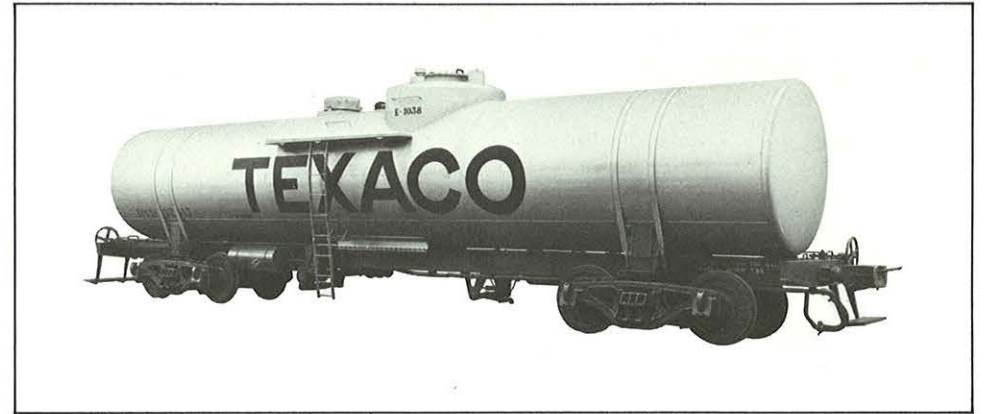
Tank cars for Ghana, with self-aligning bogies, brass bearings, vacuum brakes and link and pin couplers. Capacity: 9,200 imperial gallons. Track Gauge: 3'6". Tank Inside Diameter: 6'-10 3/4". Length over Heads: 41'-3".
