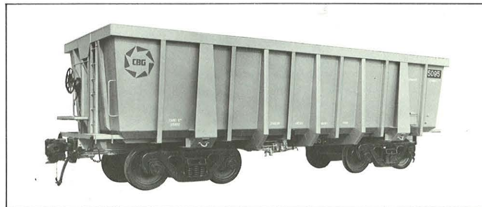
Ore cars, for Cie. de Bauxite de Guinee with Gregg-Barber stabilized bogies having Timken AP roller bearings and WABCO PAC brakes. Capacity: 75 metric tons (56 M³). Track Gauge: 1435 mm. Inside Length: 9680 mm. Inside Width: 3000 mm.
