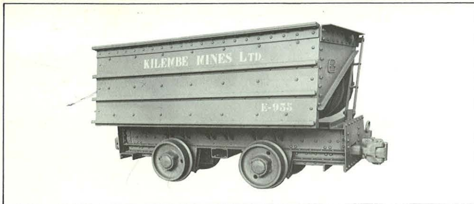
Granby-type ore cars for Uganda; sandwich floor, 2" oak between steel plates; Timken roller bearings in wheels. Capacity: 130 cubic feet. Track Gauge: 2'-6".
