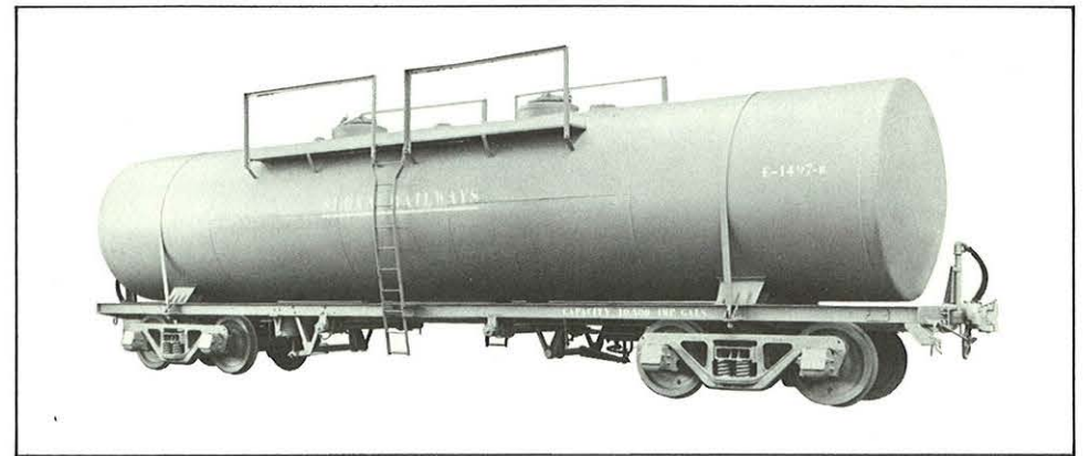
Tank cars for Sudan Railways with self-aligning bogies and vacuum brakes. Capacity: 10,500 imperial gallons. Track Gauge: 42". Tank Inside Diameter: 7'-5 3/4". Length over Heads: 40'-8".
