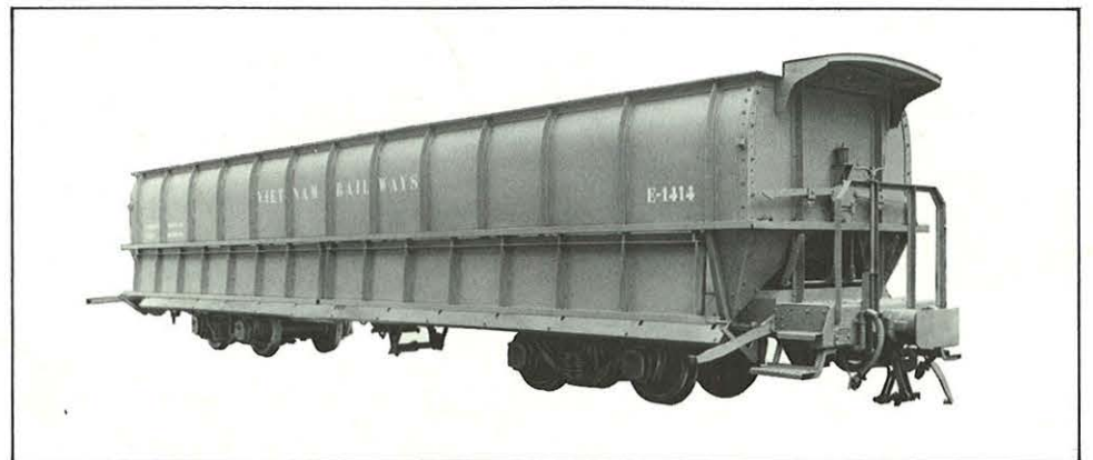
Gable-bottom coal cars; Gregg-Barber stabilized bogies with Unit brake beams. Capacity: 30 metric tons. Track Gauge: 1 meter.
