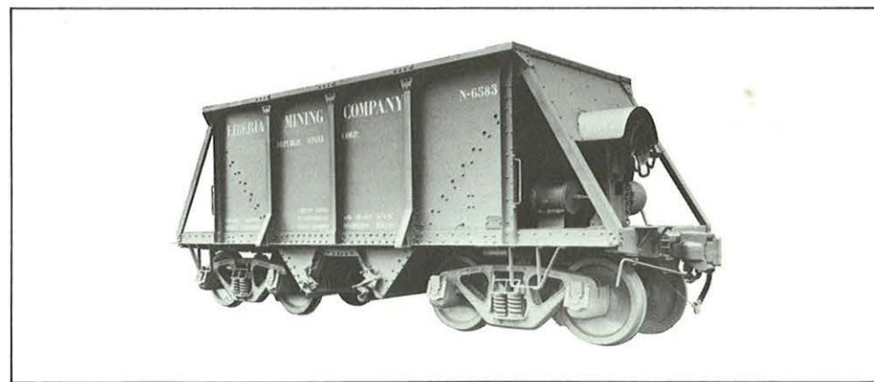
Twin-hopper iron ore cars for Liberia; Gregg-Barber stabilized bogies with Unit brake beams and brass bearings. Capacity: 50 metric tons — 589 cubic feet. Track Gauge: 3'-6".
